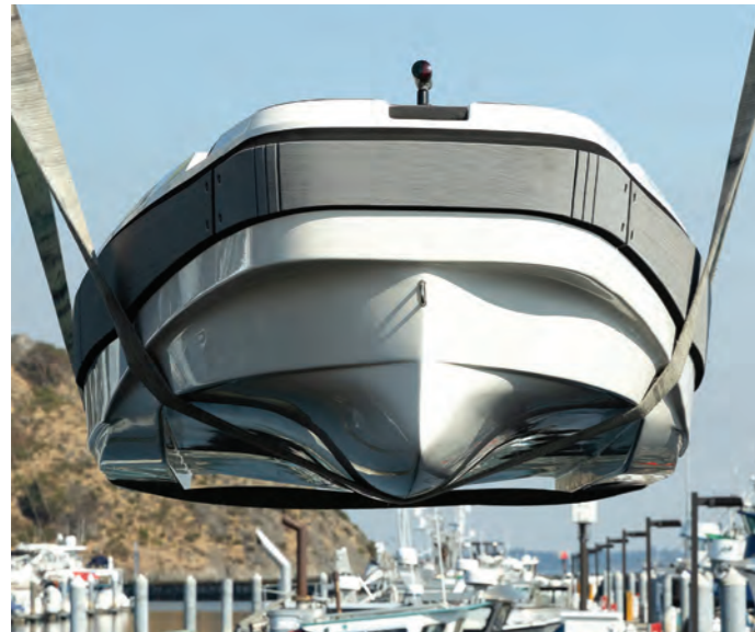
Carbon Cat's unique hybrid hull form combines a narrow entry forward with wide hulls aft that improve performance and stability.
