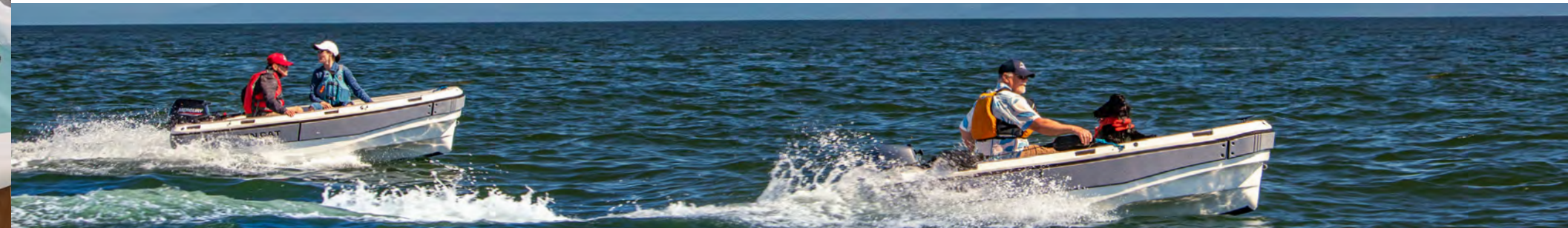
Testing T11 with 325lb weight, drain plug open, and all three hull air chambers flooded.
