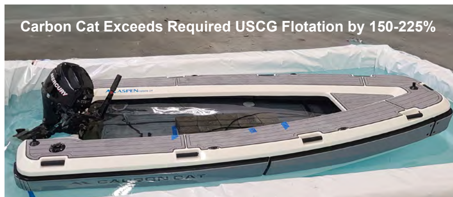
Testing T11 with 325lb weight, drain plug open, and all three hull air chambers flooded.
